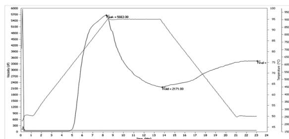
Figure 1. Gelatinisation profile of gathotan flour, showing peak viscosity of 5663.00 cP and viscosity at holding of 2172.00 cP
